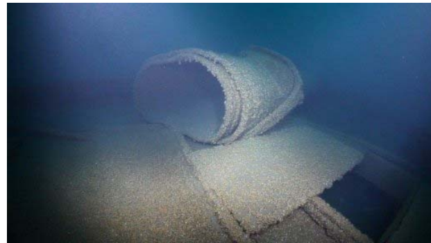
The ship's smokestack toppled on its side
